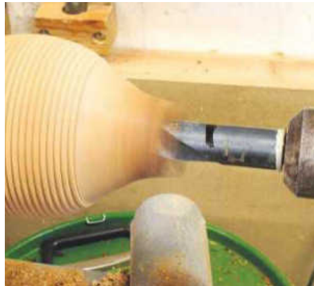
STEP 12. Whenever you are working blind inside a piece, I recommend drilling a depth hole; this will allow the tool to work from the centre out without having to worry about removing the slow timber in the middle
